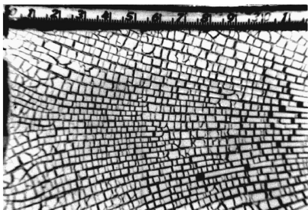
FIG. 2. The crack pattern formed in a directional drying experiment. The substrate was treated with teflon, and a sharp drying front moved front left to right across the layer, leaving behind oriented primary cracks. The rungs of the ladderlike pattern are secondary cracks. The front speed was 1.2 \text{ mm/h} . Near the middle of the picture, the depth of the layer suddenly increased by about 50%, but no change in the average spacing is evident. This illustrates the weak depth dependence and hysteretic nature of crack spacings on slippery substrates.
